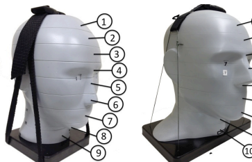
Figure 1. Child (left) and adult (right) dosimetry phantoms
