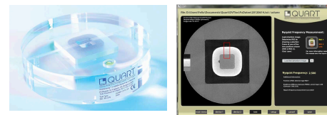
Figure 2. QUART phantom and analysis software display
